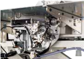
Automatic bobbin-thread winding and feeding unit
