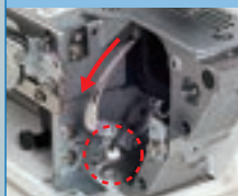
Simple looper threading
